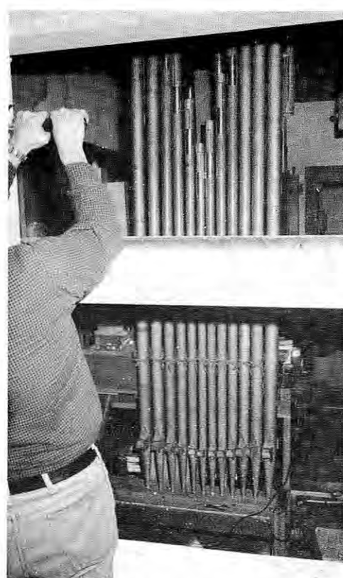
RATHER than negotiate curved stairway into chamber, it was decided to remove organ through swell shade opening. The 8 foot Salicional is seen as swell shades are taken out.
